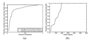
Figure 11: (a) The fraction of Web pages covered by the most common hash value in each campaign. The two curves are presented in an ascending order independently (fmax) is always 1). (b) The ratio of the average hash value occurrence within a campaign to the occurrence across all campaigns.
